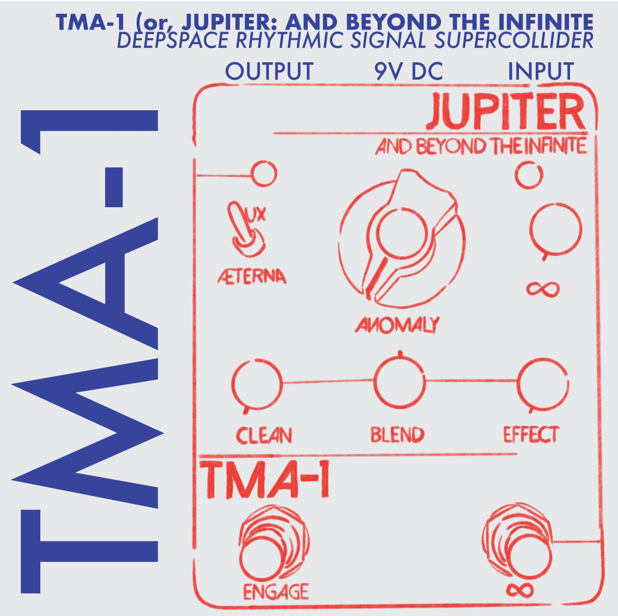
Engage: Toggles effect on/off (Bypass) Infinity Switch (∞): Toggles modulation crosstalk (no effect in bypass) Infinity Knob (∞): adjusts level of ring-mod crosstalk Anomaly knob: Sets frequency of the carrier oscillator Lux Mode: Analog carrier modulates the input signal Aeterna Mode: Input signal modulates doubled carrier frequency Mixer section: Independent controls for effected and dry signal by Discomfort Designs
